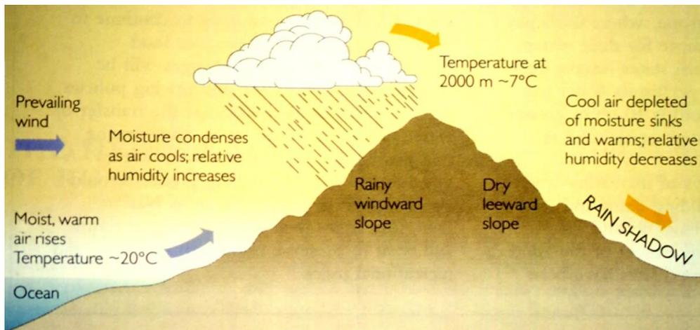
Hydrologists have long recognized that clouds dispel greater amounts of moisture over highland areas, due to a phenomenon known as “*orographic lifting*” (shown in the above diagram). In such situations we may observe levels of precipitation two to three times as high in the higher elevations and “rain shadows” develop in areas down-wind of such highlands, which receive almost no
